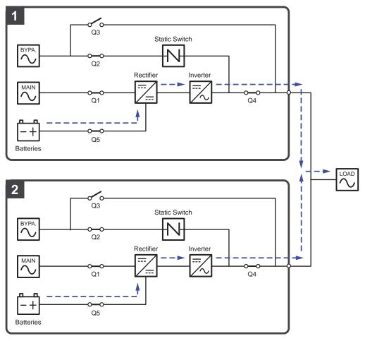
(Figure 3-23: Battery Mode Diagram\_ Dual Input Parallel Units)
