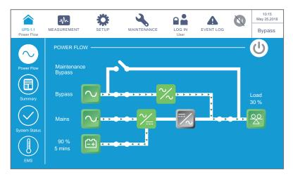
(Figure 6-54: Bypass Mode Screen)
