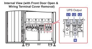
(Figure 2-9: Wiring Terminals\_ UPS Output)
