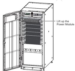
(20 ~ 120kVA UPS Internal View with front Door Open)
