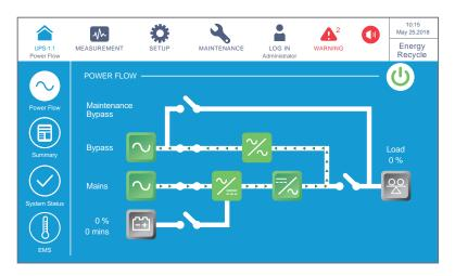
(Figure 6-44: Energy Recycle Mode Screen)
