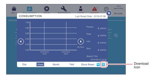
2 Tap one of the kWH Statistics Sheet Tabs to download the corresponding column chart and statistical data of a specific time scale (Day/ Week/ Month/ Year/ Since Reset).
