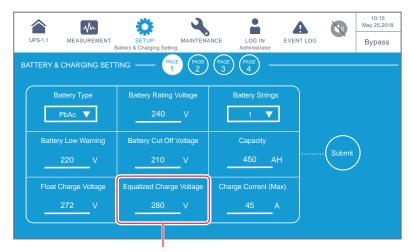
Whether it is 'Equalized Charge Voltage' or 'Restore Voltage' shown in this column, it is determined by 'Battery Type'. Please refer to the table shown in Page 7-47 for more information.
