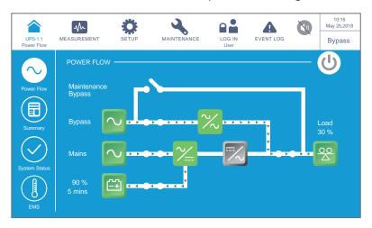
(Figure 6-47: Bypass Mode Screen)
