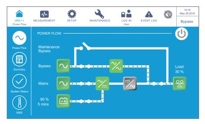
(Figure 6-51: Bypass Mode Screen)
