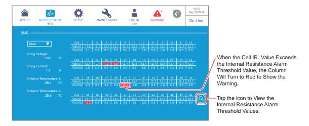
Press the icon ( ), and you can view the **Internal Resistance Alarm Threshold** values of each cell shown in the figure below.
