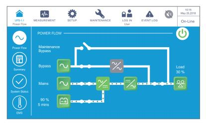
(Figure 6-20: On-Line Mode Screen)
