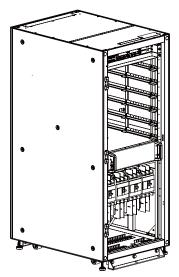
(Figure 4-22: Cabinet Internal View after Removal of Every Power Module Slot's Cover and Wiring Panels)
