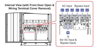
(Figure 5-8: Wiring Terminals\_ AC Input & Bypass Input)
