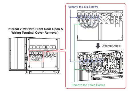
(Figure 5-7: Remove the Six Screws & Three Cables)
