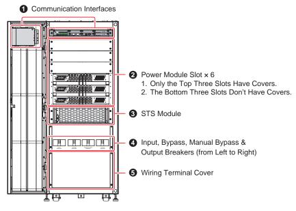
(Figure 2-4: UPS Internal View with front Door Open)
