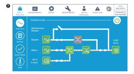
The screen above indicates that the UPS is in **Frequency Conversion** mode and the bypass output is restricted. For **Frequency Conversion** mode settings, please refer to **7.10.2 Mode Setting** and **6.2.6 Frequency Conversion Mode Start-up Procedures**.
