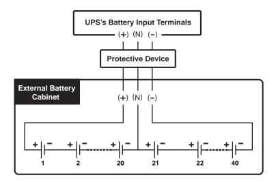
(Figure 5-20: External Battery Cabinet Connection)
