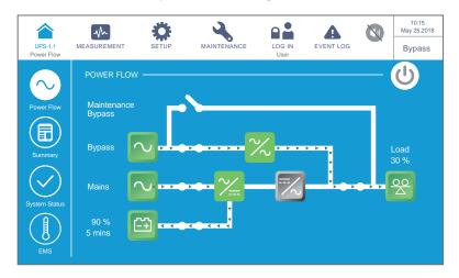
(Figure 6-64: Bypass Mode Screen)
