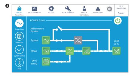
The screen above indicates that the UPS is in **Green** mode, and power supply of the loads comes from the inverter. Power modules will take turn to rest depending on the total load situation. For **Green** mode settings, please refer to **7.10.2 Mode Setting** and **6.2.7 Green Mode Start-up Procedures**.
