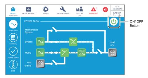
(Figure 6-67: Energy Recycle Mode Screen & ON/ OFF Button Location)
