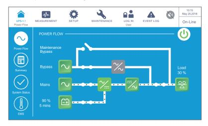
(Figure 6-5: On-Line Mode Screen)
