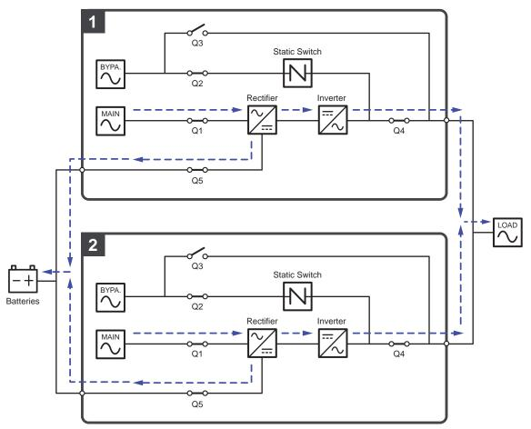
(Figure 3-29: Common Battery Diagram\_ only for Parallel UPSs Connecting to the Same External Battery Cabinet(s))
