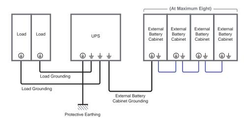
(Figure 5-16: Grounding Diagram\_ Single Unit)
