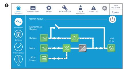
The screen above indicates that the UPS is in Bypass mode and the inverter is off.
