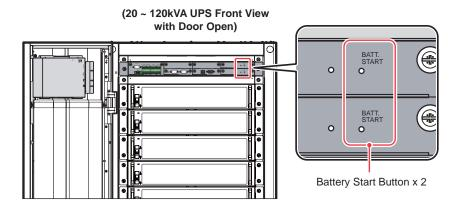
(Figure 7-2: The Position of Battery Start Buttons)
