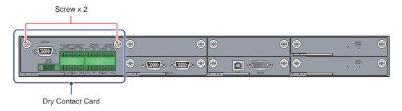
(Figure 4-5: Dry Contact Card Location)
