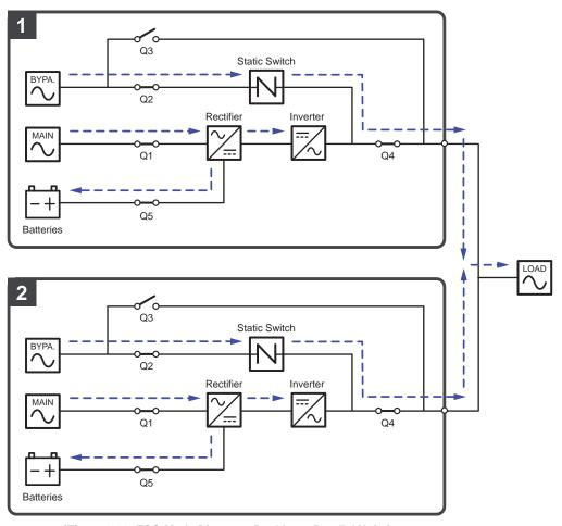
(Figure 3-26: ECO Mode Diagram\_ Dual Input Parallel Units)
