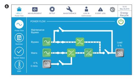
The screen above indicates that the UPS is in **Energy Recycle** mode. The output power will be recycled to the main input without being sent to the loads and the aging test could be conducted. For **Energy Recycle** mode settings, please refer to **7.10.2 Mode Setting** and **6.2.8 Energy Recycle Mode Start-up Procedures**.
