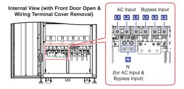
(Figure 2-7: Wiring Terminals\_ AC Input & Bypass Input)
