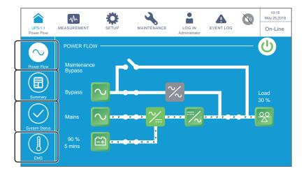
1. Tap the icon to check the UPS's power flow diagram. Please refer to the figure below.
