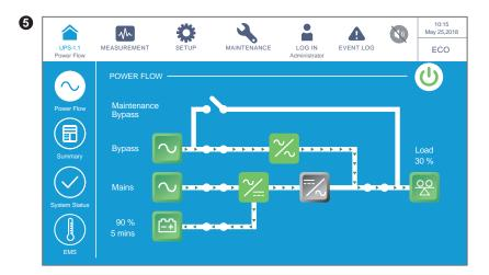
The screen above indicates that the UPS is in **ECO** mode. The inverter is in the ready-to-power-on status, and the power supply of the loads comes from the bypass. For **ECO** mode settings, please refer to **7.10.2 Mode Setting** and **6.2.5 ECO Mode Start-up Procedures**.
