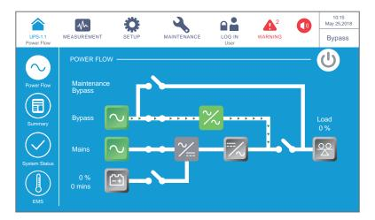
(Figure 6-69: Bypass Mode Screen)
