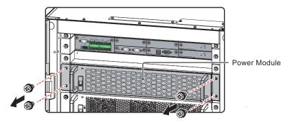
(Figure 5-45: Remove the Four Screws)
