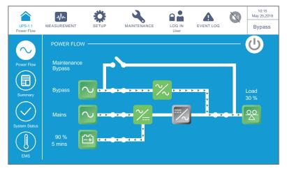
(Figure 6-13: Bypass Mode Screen)
