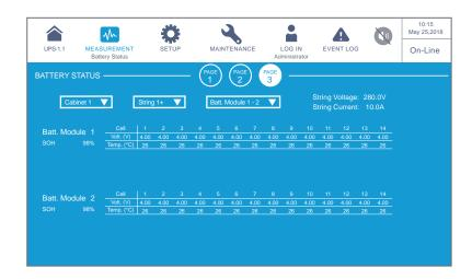
After entering the screen shown above, you can use the three drop-down lists in the upper left corner to choose the **Cabinet, String**, and **Battery Module** to view the corresponding **String Voltage**, **String Current**, battery module's **SOH** (State of Health) and battery cell's **Voltage** and **Temperature**.
