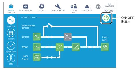
(Figure 6-45: On-Line Mode Screen & ON/ OFF Button Location)
