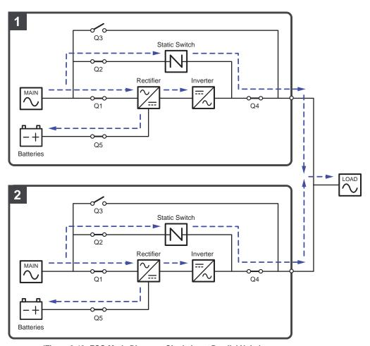
(Figure 3-13: ECO Mode Diagram\_ Single Input Parallel Units)
