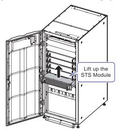
(Figure 5-34: Lift up the STS Module)
