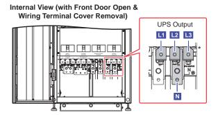
(Figure 5-10: Wiring Terminals\_ UPS Output)
