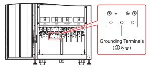
(Figure 2-10: Wiring Terminals\_ Grounding)
