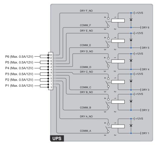
(Figure 4-9: Output Dry Contacts Design)
