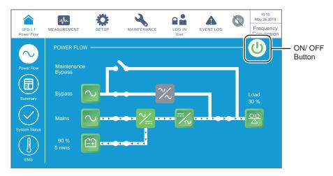
(Figure 6-57: Frequency Conversion Mode Screen & ON/ OFF Button Location)
