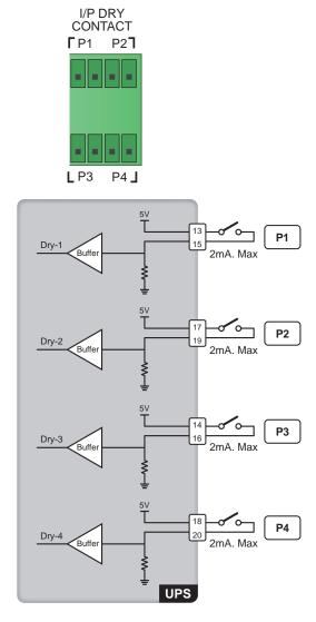
(Figure 4-10: Input Dry Contacts Design)
