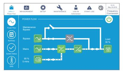
(Figure 6-32: Frequency Conversion Mode Screen)
