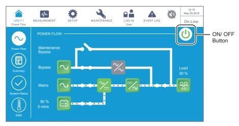
(Figure 6-14: On-Line Mode Screen\_ User Login & ON/ OFF Button Location)
