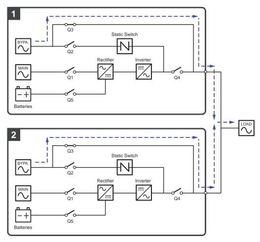
(Figure 3-25: Manual Bypass Mode Diagram\_ Dual Input Parallel Units)
