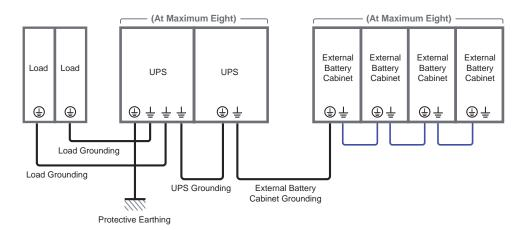
(Figure 5-18: Grounding Diagram\_ Parallel Units)
