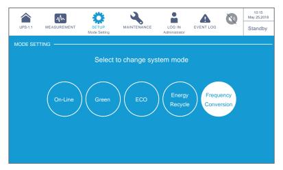
(Figure 6-30: Select Frequency Conversion Mode)
