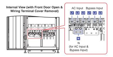
(Figure 5-6: Wiring Terminals\_ AC Input & Bypass Input)
