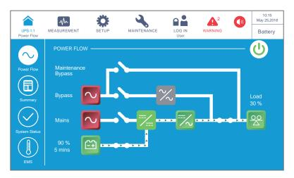
(Figure 6-9: Battery Mode Screen)
