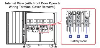
(Figure 2-8: Wiring Terminals\_ Battery Input)
