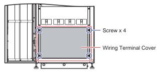
(Figure 5-5: Wiring Terminal Cover & Screw Location)
