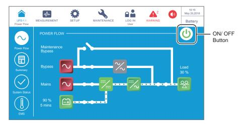
(Figure 6-48: Battery Mode Screen & ON/ OFF Button Location)
