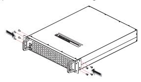
(Figure 5-39: Install the Two Bracket Ears)
