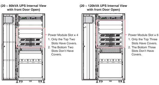
(Figure 5-40: Power Module Slot's Cover Location)
