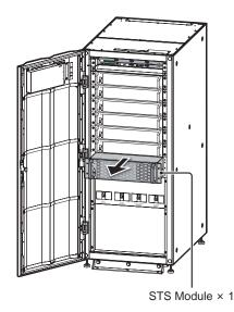
(Figure 5-33: Remove the STS Module)
